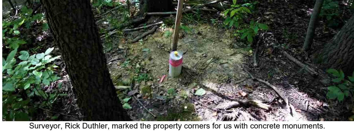
Surveyor, Rick Duthler, marked the property corners for us with concrete monuments.
